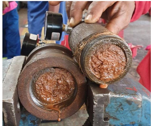
**Fig. 9** Cross-sectional view of the chamber containing condensate soaked plugged packed sand after testing
